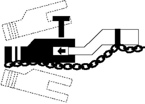
The machine's frame must be level for ease of towing, as well as operator and crew safety. The hitch should be located so that the truck bed overhang will not interfere with the extended load tray.
