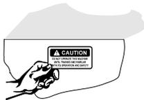
Carefully read all safety messages in your operations manual and on your Power Mulcher. Keep safety signs in good condition. Replace missing or damaged safety signs. Be sure new equipment components and repair parts include current safety signs and safety guards. Replacement safety signs and guards are available from your Reinco dealer or directly from Reinco.
