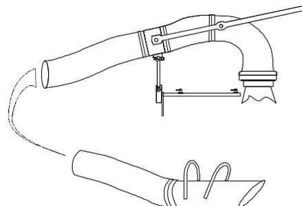
Mulching can now be started. Adjust throttle to desired speed and begin feeding untied mulch bales while a second person directs discharge at the hose end.
