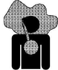
The electrical systems of engines can be a source of high voltage. Never touch electrical wires or components when engine is running. Never attempt to start the engine by shorting across the starter solenoid.
