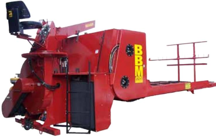
The BBM200 Big Bale Mulcher is our most productive Straw Blower. The large stored bale capacity and its ability to process and discharge large volumes of material make this unit the contractor's ideal choice in high production mulching equipment. Powered by a 200 horsepower Caterpillar diesel engine, the BBM200 will discharge straw up to a distance of 120 feet in still air at a discharge rate of 30 tons per hour.
